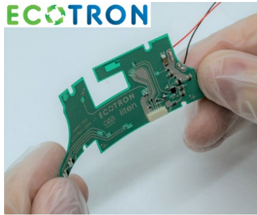
ECOTRON: Flexible, printed PCB for on-body subcutaneous drug delivery system © CEA LITEN France (Image in higher resolution)
