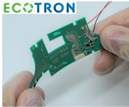
ECOTRON: Flexible, printed PCB for on-body subcutaneous drug delivery system/ Flexible, gedruckte Leiterplatte © CEA
